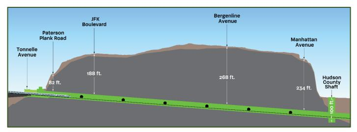
The Project includes boring **two parallel tunnels approximately 5,100-feet long** with an inside diameter of 25 feet 2 inches and **six cross passages**, as well as furnishing and installing a concrete tunnel lining with waterproofing membrane.
